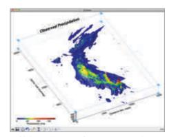
In this image, IDL was used to create a contour image of the observed levels of precipitation on the plains of Texas. Labels have been used to create an image title and identify axes. Additionally, a color legend was created and labeled to show how different colors correspond to precipitation amounts.
